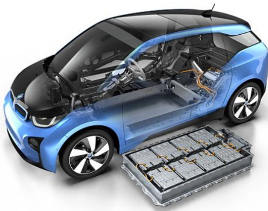
Picture: Battery package of BMW i3- No loss of interior space if constructed from the outset as an e-car.
