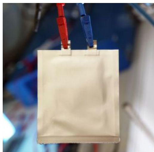
Thin film battery with printed polymer-based electrode. (©Jan-Peter Kasper/FSU)
