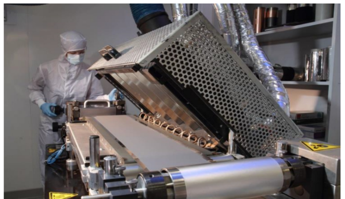
Figure: Coating machine used at CEA-Liten for Gen-1B formulation selection.
